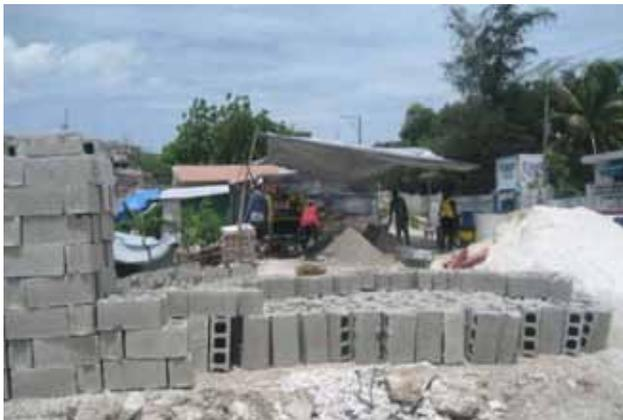
Block being manufactured with little quality control, poor curing, and inferior raw materials (sand/aggregate). If provided with properly graded and tested raw materials, clean water and education about proper curing and handling, strength of the block can be greatly improved at minimal expense.
