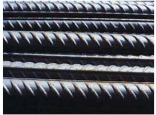
Here is a photo of “deformed rebar” showing ribs which allow the concrete to grip the steel for structural integrity. Unfortunately much of the rebar used in Haiti is smooth and therefore the concrete fails when the bar breaks away from the concrete. What is the cost of proper rebar? What is the cost of not using the right materials?
